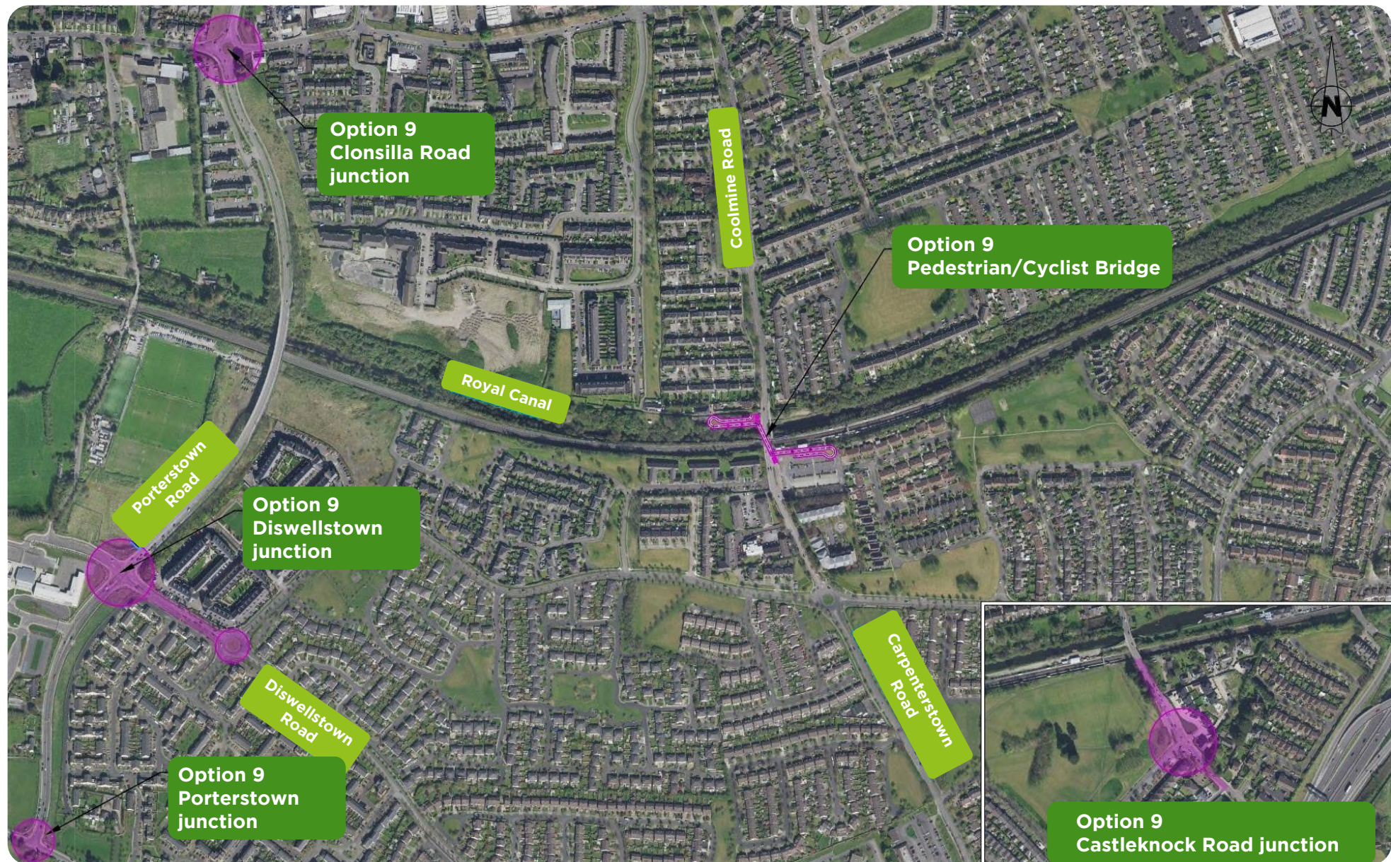
Graphic of Preferred Option for road junction improvements to facilitate Coolmine level crossing replacement
